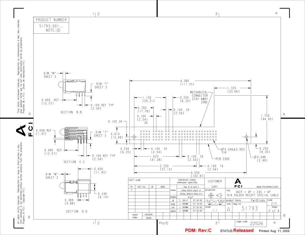
1|2 3 | DIM "M" DIM "T" PLATING LTEM MATING TAIL CONTACT FOR NO. LENGTH LENGTH TYPE MATING +/-.0|0 +/-.010 [N/A] 0.135 [3.43] SIGNAL 6 N/A30 u′′ [.76um]Au 0.135 6 N/A[N/A][3.43] SIGNAL 30 u′′ [.76um]Au [.76um]Au 0.135 [3.43] G 6 N/A [N/A]SIGNAL 30 u′′ N/A [N/A] 0.135 [3.43] SIGNAL 30 u′′ [.76um]Au 6 Н [2.34] 0.135 30 u′′ PC 0.092 [3.43] POWER [.76um]Au
